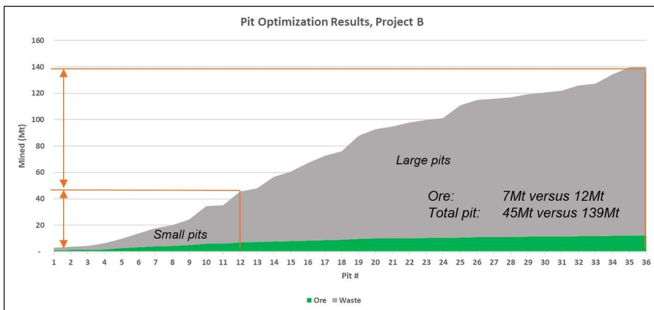
Figure 5 ore and waste mined for Project B
