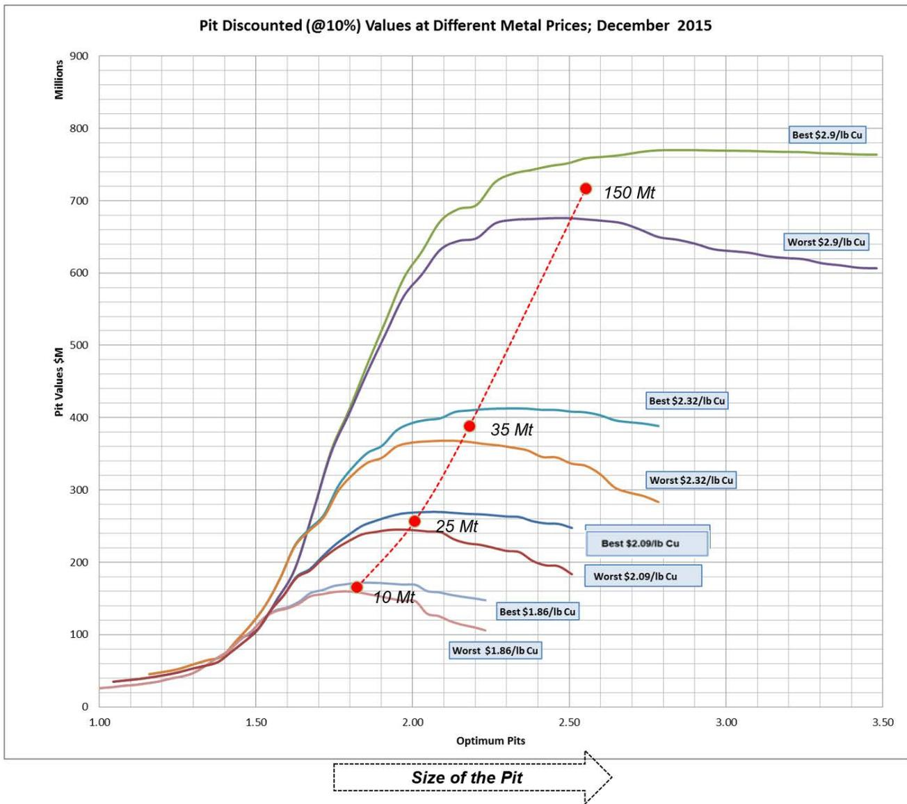
Figure 1 discounted value for different sizes of pits
