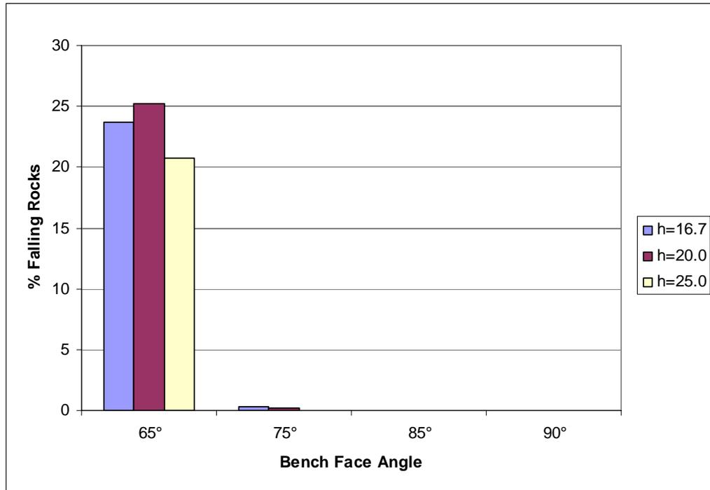
**Figure 20: BSA=46°. Percentage of falling rocks that reach the base of the bench stack**
