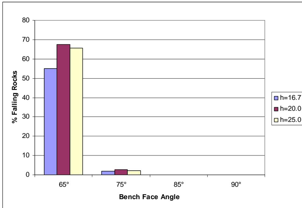
**Figure 21: BSA=52°. Percentage of falling rocks that reach the base of the bench stack**
