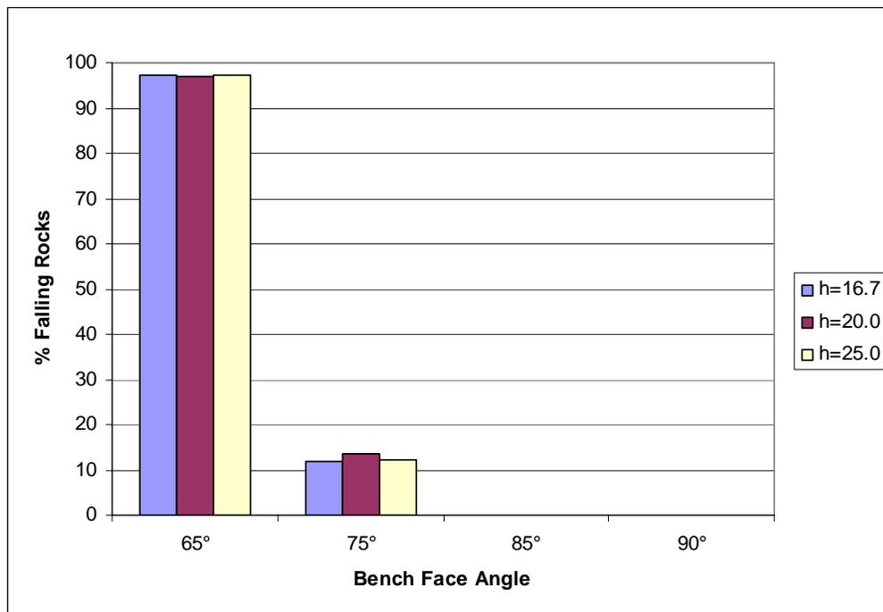
**Figure 22: BSA=58°. Percentage of falling rocks that reach the base of the bench stack**
