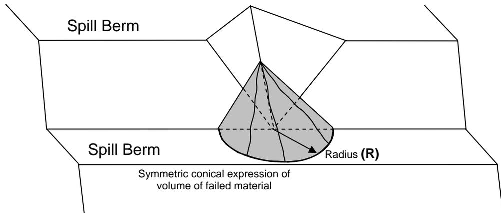
**Figure 11: 3-D illustration of symmetric conical distribution of failed material on a spill berm**
