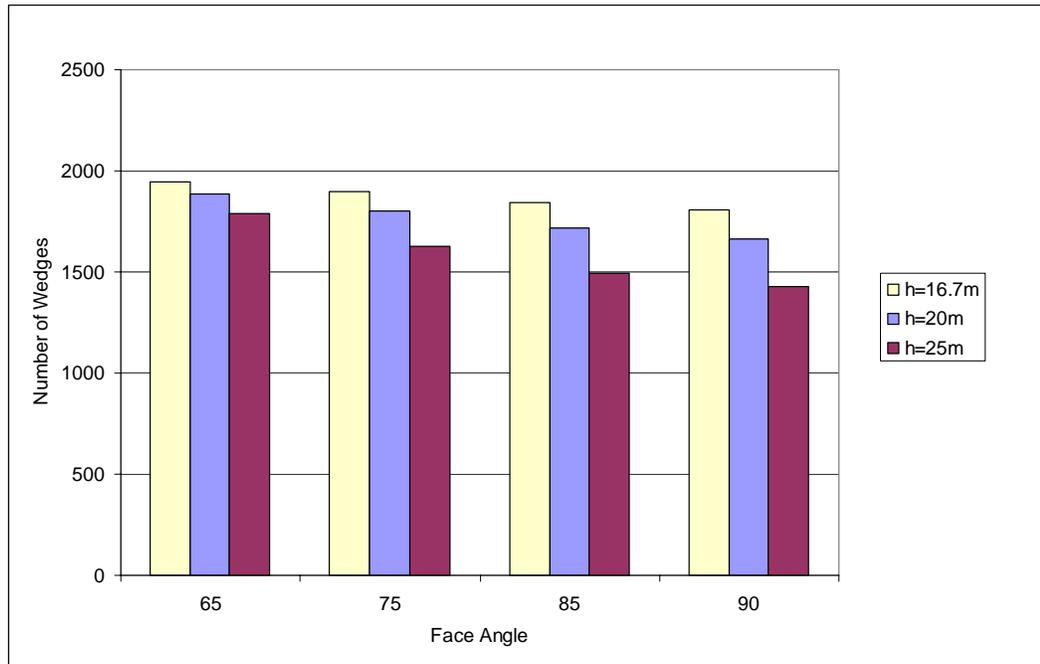
**Figure 14: BSA = 52°. Number of wedge failures that will result in spillage of material from the berm**
