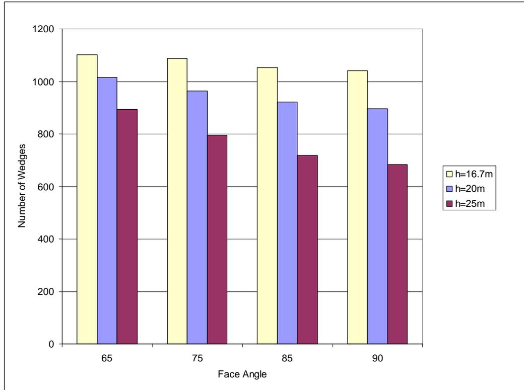
**Figure 13: BSA = 46°. Number of wedge failures that will result in spillage of material from the berm**
