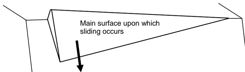
**Figure 3: 3-D illustration of failure of a highly asymmetric wedge approximating planar failure**
