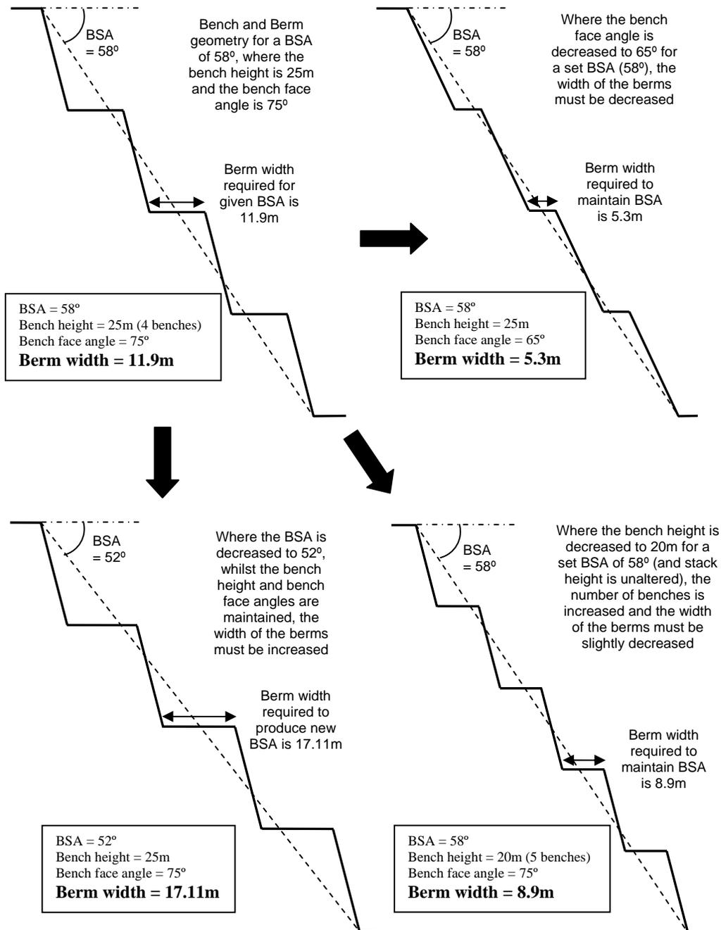
**Figure 10: Effect of variation in bench height, bench face angle and BSA on the limiting spill berm width to be entered into wedge failure volume analysis**
