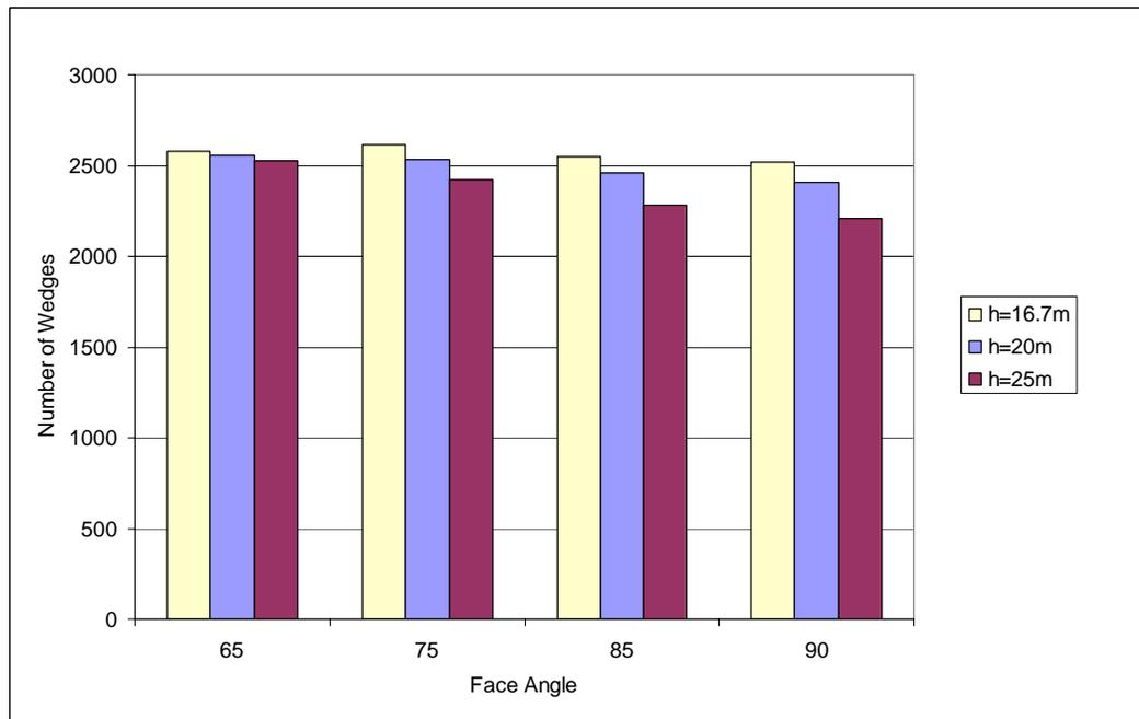
**Figure 15: BSA = 58°. Number of wedge failures that will result in spillage of material from the berm**
