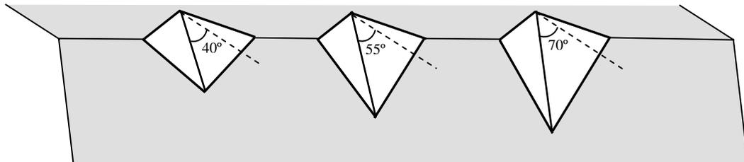
**Figure 4: 3-D illustration to show variations in steepness of plunge of the line of intersection for joints sets forming wedges**
