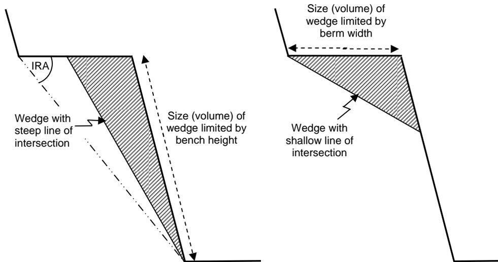
**Figure 8: Sectional illustration of the limitations of bench height and berm geometry width on wedge size**
