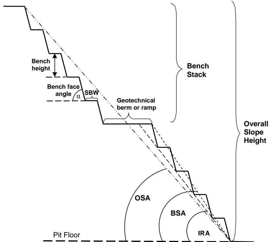
Where: IRA = Inter Ramp Angle measured from toe to toe; BSA = Bench Stack Angle, measured from toe to crest;
