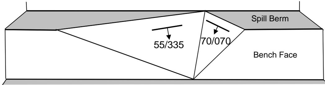
**Figure 5: 3-D illustrative example of two joints of different dip/dip direction combinations forming a wedge**
