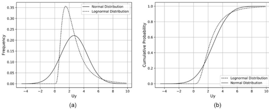
**Figure 2.** Distribution of probability (a) and cumulative probability (b) of the vertical displacement  $U_y$  for uncorrelated cohesion and friction angle using PEM and both normal and lognormal distributions.
