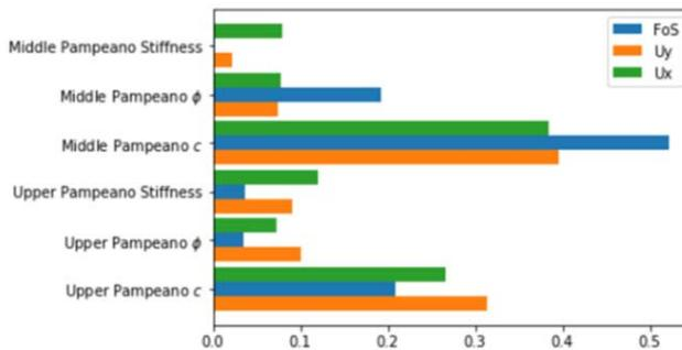
**Figure 3.** Sensitivity score plot for all the variables and the different target functions:  $FoS$ , vertical displacement  $U_y$  and horizontal displacement  $U_x$ .
