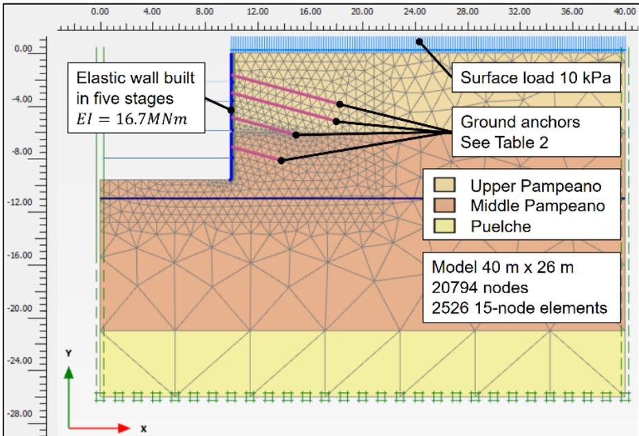
Figure 1. Geometry and finite element mesh.
