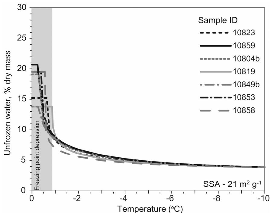
**Figure 6** Estimated unfrozen water content curves for Pogo tailings, assuming fresh pore water
