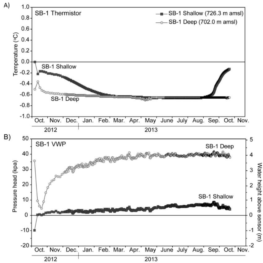
**Figure 4 Sonic borehole SB-1 shallow and deep: A) ground temperature from October 2012 to October 2013, and B) VWP pore pressure from October 2012 to October 2013**
