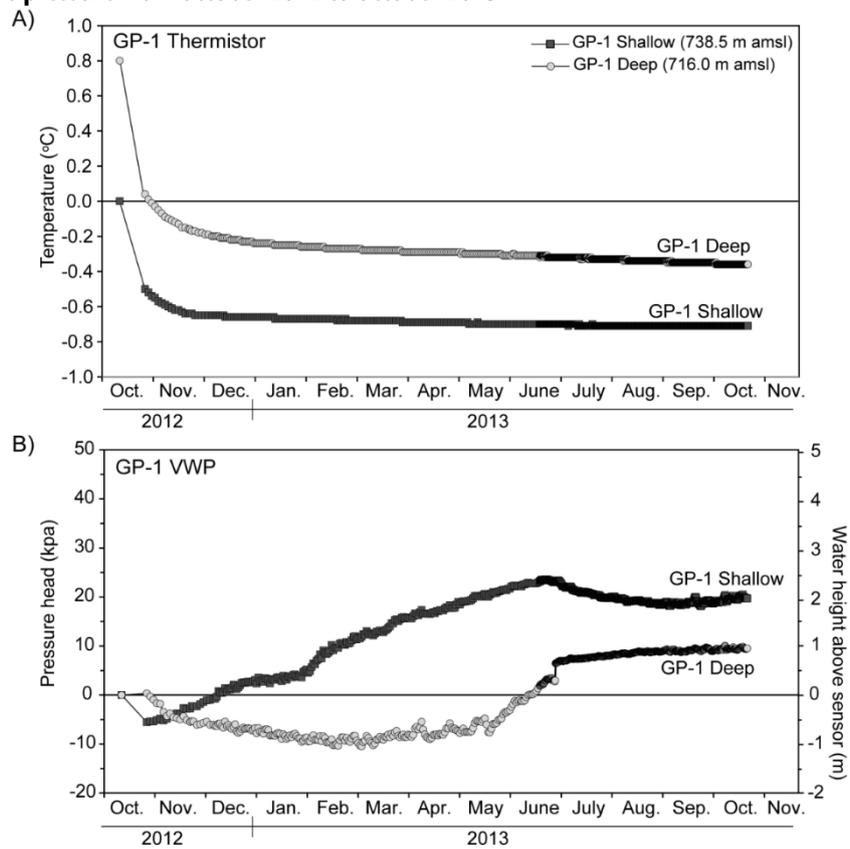
**Figure 5 Sonic borehole GP-1 shallow and deep: A) ground temperature from October 2012 to October 2013, and B) VWP pore pressure from October 2012 to October 2013**
