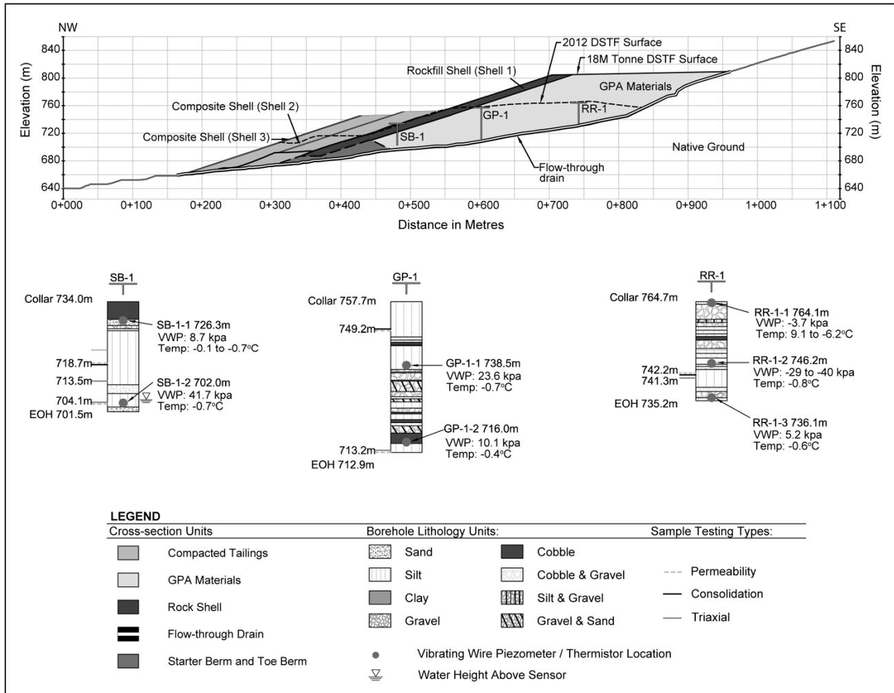
**Figure 2 Cross-section of 18 M t DSTF and generalised borehole stratigraphy at SB-1, GP-1, and RR-1 (for clarity, the stratigraphic locations of SPT and geotechnical grab samples are not shown)**
