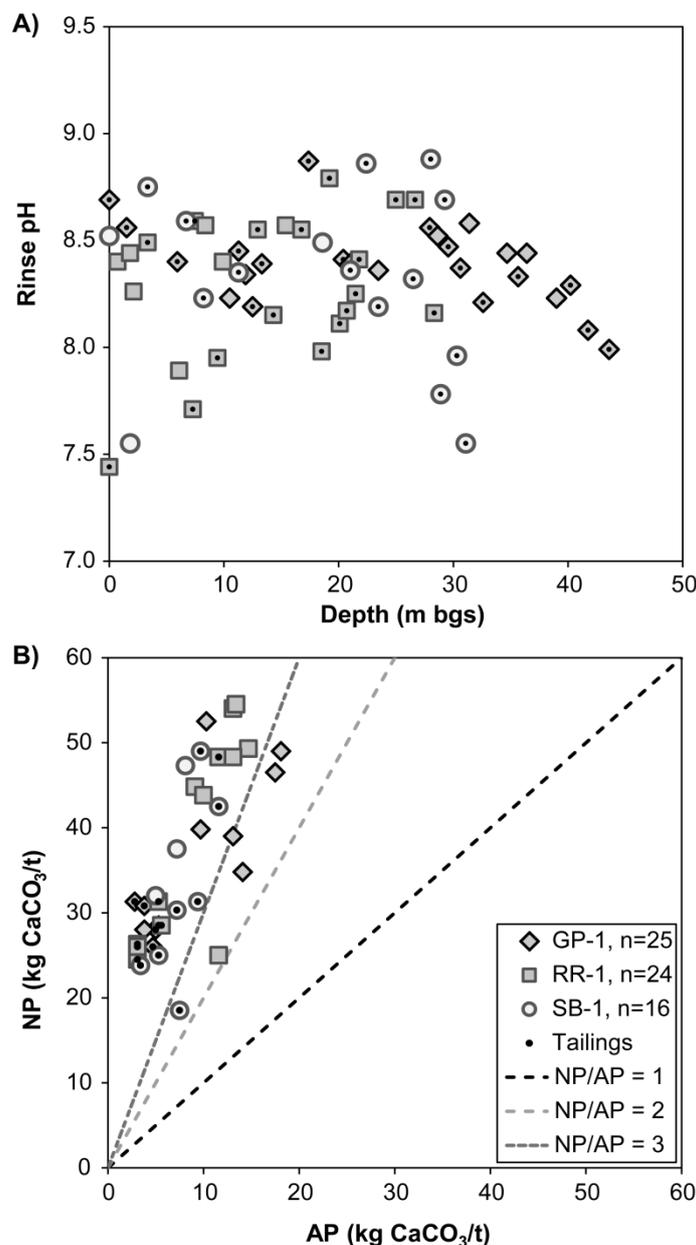
**Figure 7** A) Rinse pH versus depth and B) neutralisation potential (NP) versus acidification potential (AP) for tailings and waste rock samples recovered from boreholes RR-1, SB-1, and GP-1
