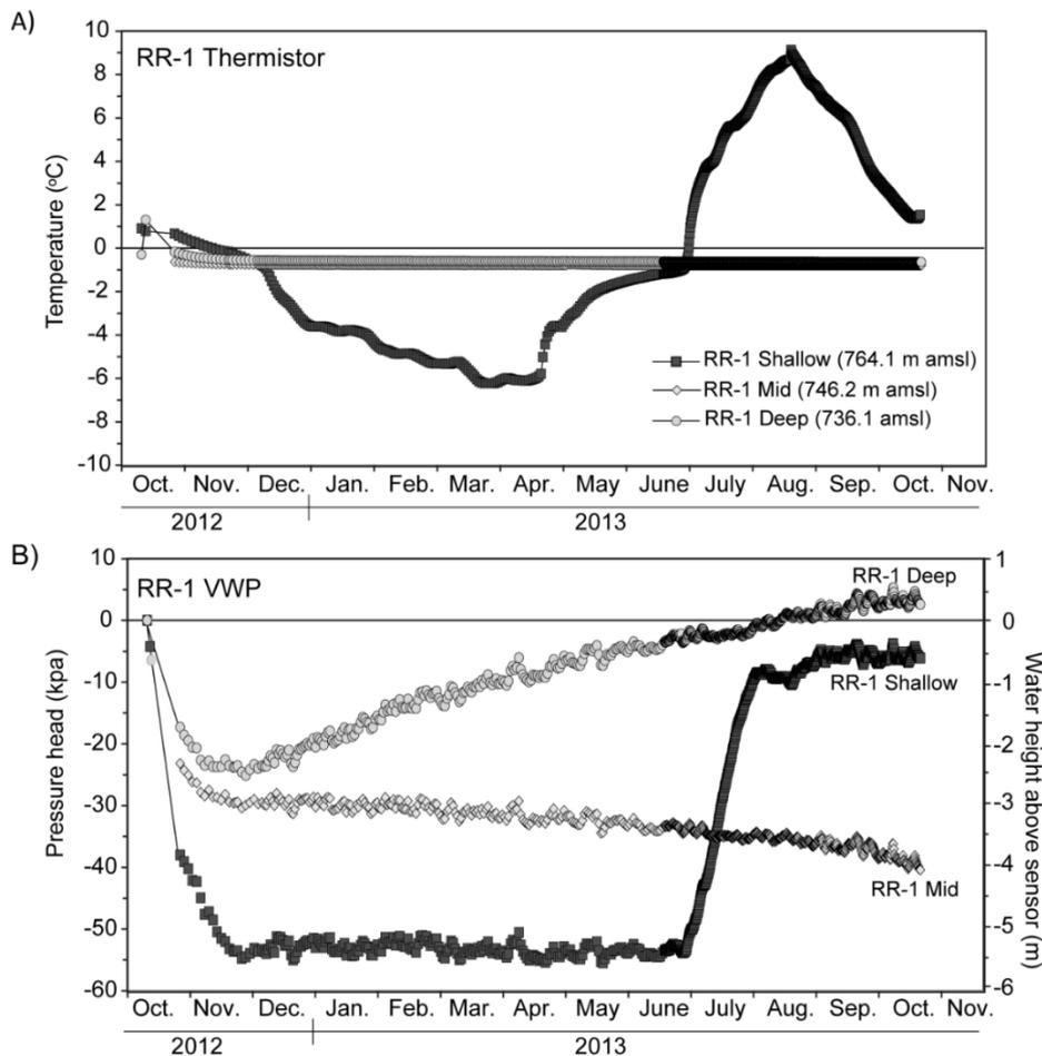
**Figure 3** Sonic borehole RR-1 shallow, mid, and deep: A) ground temperature from October 2012 to October 2013, and B) VWP pore pressure from October 2012 to October 2013
