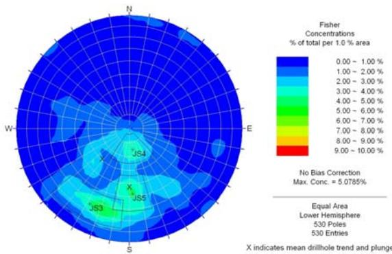
Fig. 4. Stereoplot of oriented core discontinuities from two holes drilled with inclinations towards the south and southwest.
