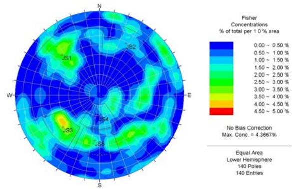
Fig. 5. Stereoplot of discontinuities obtained by cell mapping.
