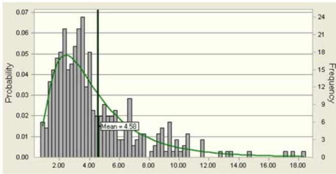
Fig. 6. Distribution of discontinuity lengths obtained from LiDAR scans.
