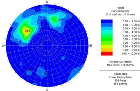
Fig. 2. Stereoplot of discontinuities obtained with LiDAR.
