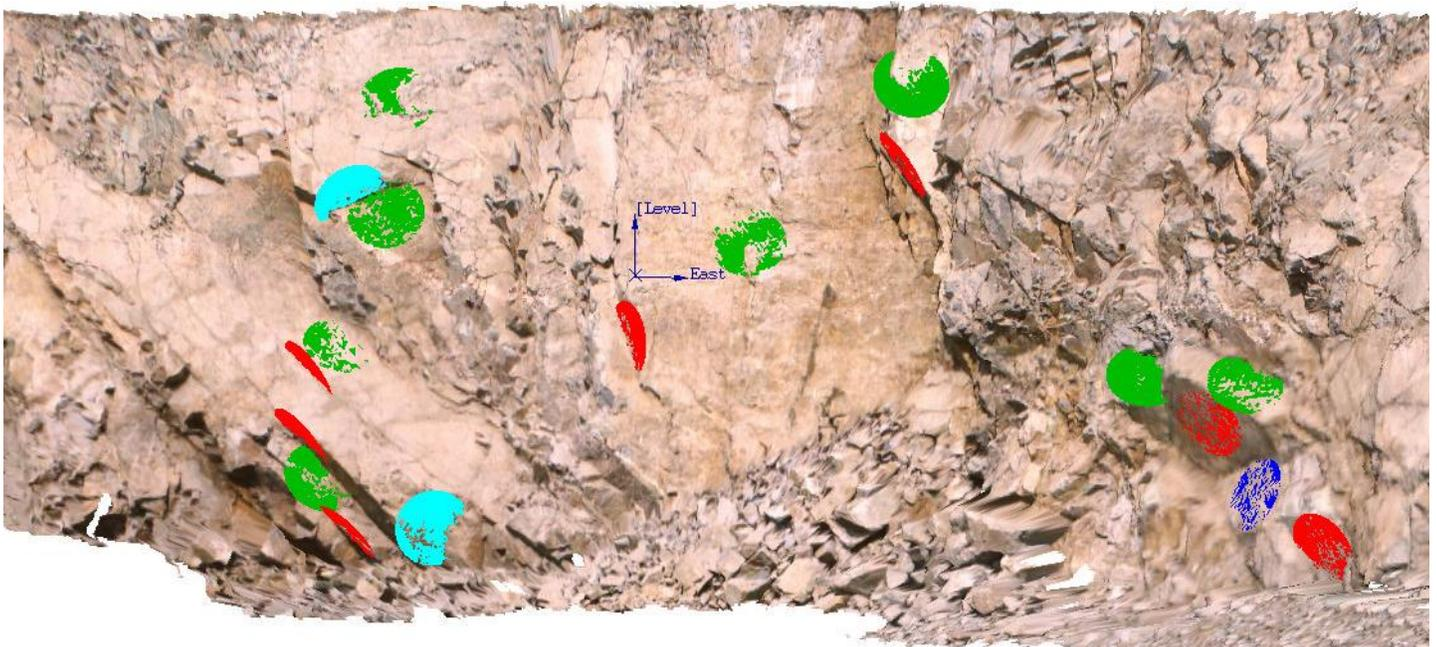
Fig. 1. Typical 3-dimensional bench face model obtained remotely using LiDAR. Digitized structures are shown as discs colored by joint set.
