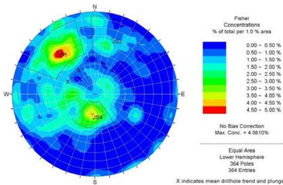
Fig. 3. Stereoplot of oriented core discontinuities from two drillholes drilled with inclinations towards the northwest.
