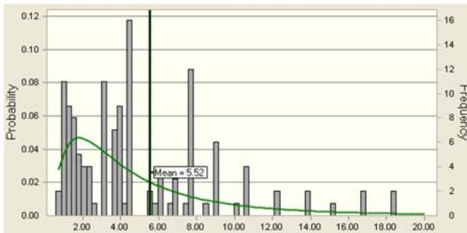
Fig.7. Distribution of discontinuity lengths obtained with field cell mapping.
