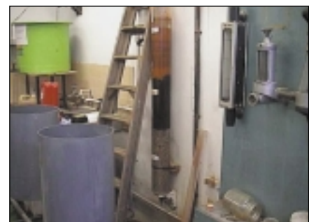
Figure 3: Laboratory reconstruction of the Pelenna SAPS
